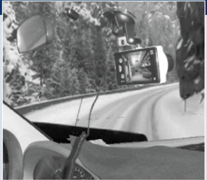
Road condition information is directly reported from the windshield of a snow plow into PennDOT's Road Condition Reporting System and then into other applications, such as 511PA.
